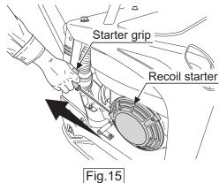
3 After the engine has started, warm up the engine at low speed for 2 to 3 minutes. This is especially important in cold weather.
