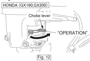
8 After the engine has started, warm up the engine at low speed for 2 to 3 minutes. This is especially important in cold weather.
