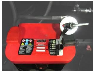
Battery switch mounted on the battery itself
