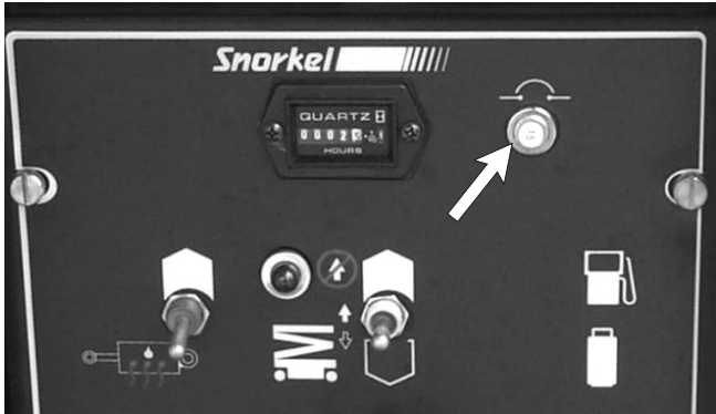
Figure 5.4 - Main Circuit Breaker
