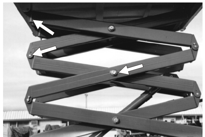
Figure 7.19 - Structural Damage and Welds
