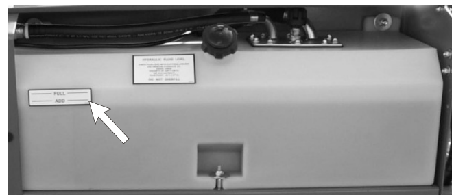
Figure 4.4 - Hydraulic Oil Level
