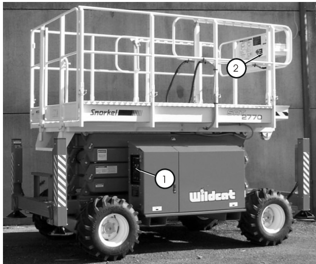
Figure 6.1 - Control Box Locations
