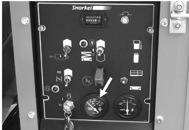
Figure 4.1 - Water Temperature Gauge
