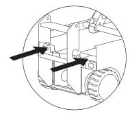
Position the forklift forks in position with the forklift pockets.
