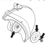
Do not use warped, notched, indented or dirty flange washers. Do not use different dimensions of flange washers.
