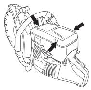
Check the air filter and replace if necessary.
