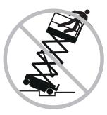
Do not drive the machine on or near uneven terrain, unstable surfaces or other hazardous conditions with the platform raised.
