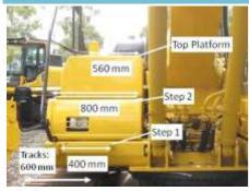
**Details** Track width on right hand side (i.e. maintenance) access system is 600 mm compared to the maximum stairways width of 800 mm.
