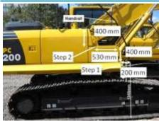
Details Step 1 dimensions on right hand side (i.e. maintenance) access system is 200 mm by 400 mm. Step 2 dimensions on right hand side (i.e. maintenance) access system is 530 mm by 400 mm.
