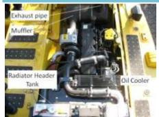
**Details** Exhaust pipe, muffler, radiator header tank and oil cooler.
