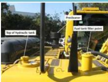
**Details** Precleaner, fuel fill point and top of hydraulic tank partially obstruct walkways on the top platform of the machine.
