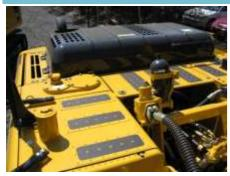
Details Top platform of machine has no guardrailing and is a work area for refuelling, topping up hydraulic oil, fuel/coolant filter replacement, checking levels of engine and swing gear box oils,maintaining beacon lighting and cleaning rear cabin window. Tracks are a work area for cleaning front and side cabin windows.
