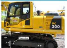
**Details** Vertical distance between ground and track step is 530 mm. Vertical distance between track and cabin floor is 470mm.
