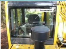
**Details** Emergency egress located near engine compartment.
