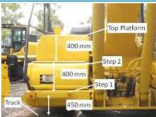
Details Vertical distance between track and step 1 on right hand side (i.e. maintenance) access system is 450 mm.
