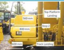
**Details** Top platform landing width on right hand side (i.e. maintenance) access system is 560 mm compared to the maximum stairways width of 800 mm.
