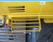
**Details** Dimensions of openings in Step 1 floor on right hand side (i.e. maintenance) access system are 390 mm x 50 mm.
