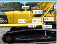
**Details** Rises on right hand side (i.e. maintenance) access system vary between 400 mm to 450 mm. Goings on right hand side (i.e. maintenance) access system vary between 200 mm to 530 mm.
