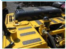
**Details** Top platform of machine has no guard railing.
