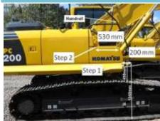
Depth of step 1 on right hand side (i.e. maintenance) access system is 200 mm.
