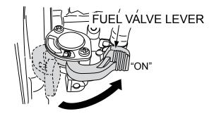
Figure 10. Fuel Valve Lever
