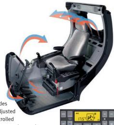
The high performance air conditioning provides an air flow which is adjusted and electronically controlled for the conditions. Five operating modes enable even the most demanding operator to be satisfied.
